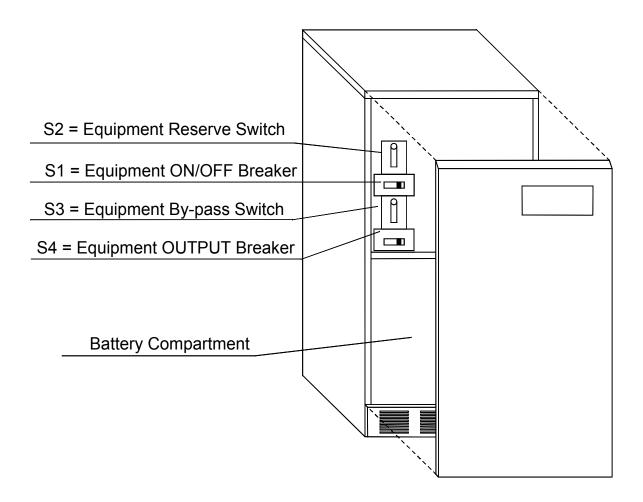
Figure 18 - 24 – 12/18/24kVA: Switches and Breakers
